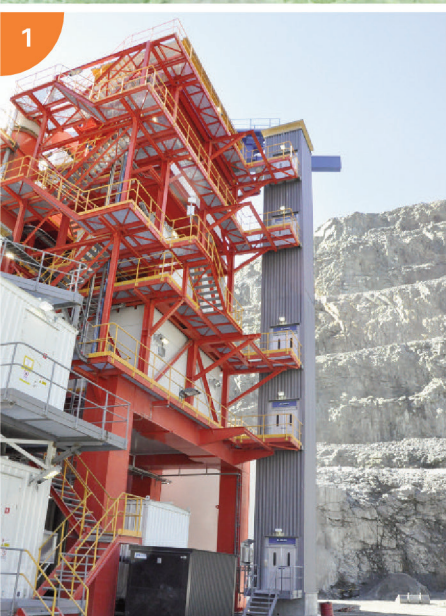
In-pit Crusher Elevator: ALIMAK SE 1000 Capacity: 1000 kg Lifting height: 24 m
